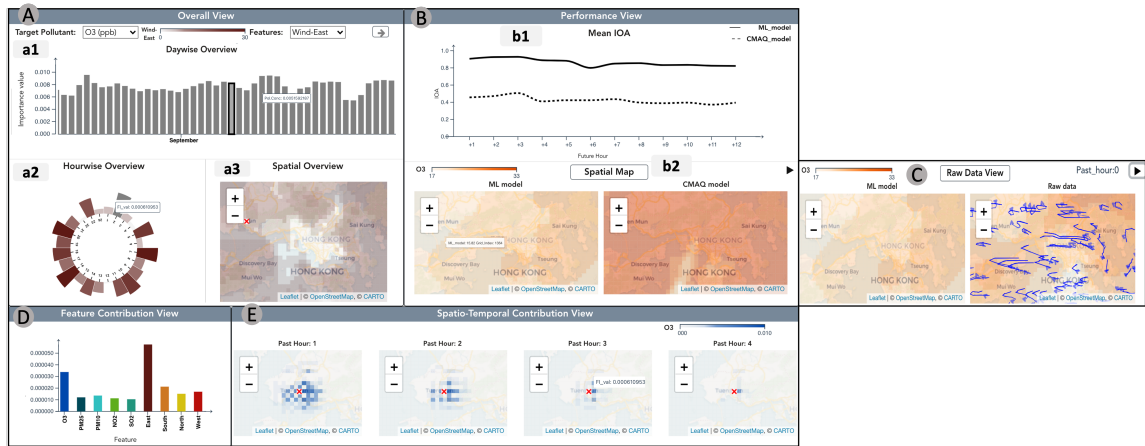
Fig. 5. ML model’s learning during extreme weather conditions. Daywise (a1), Hourwise (a2), and Locationwise (a3) feature contributions of the selected pollutant. Performance View showing Mean_IOA (b1) and Spatial Map (b2) of ML and simulation model. Raw data View (c) showing wind trajectories. Feature Contribution View (d) showing the overall feature importance of the selected instance, and Spatio-Temporal Contribution View (e) showing the grid level contribution.
